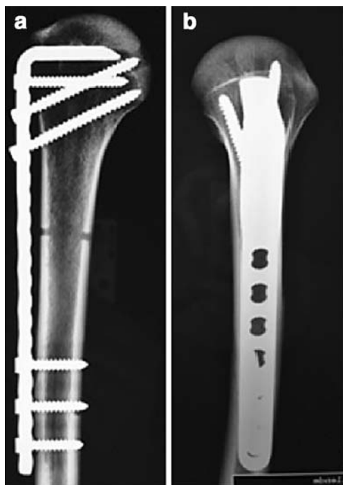
Fig. 1 Anteroposterior (a) and lateral (b) views of cadaveric bone with locked 90° blade plate showing divergent locked screw orientation into the humeral head
